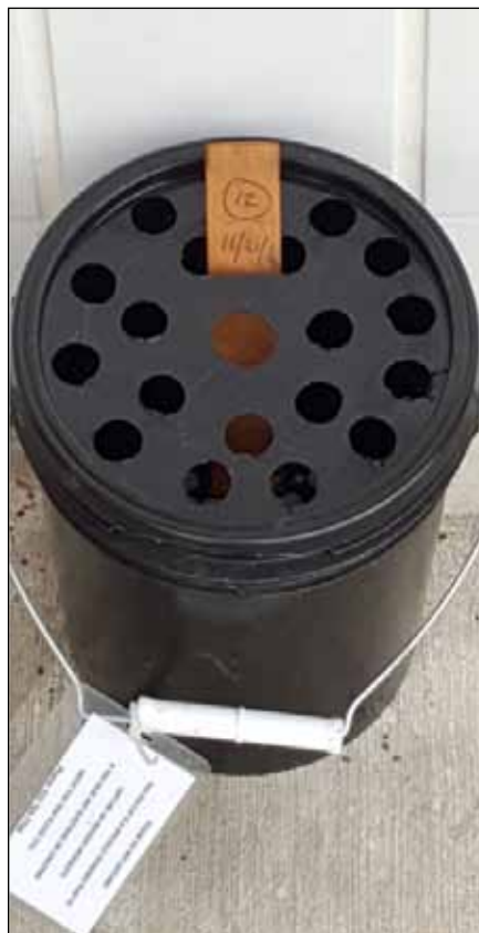
Figure 1. Assembled ovitrap bucket with oviposition substrate. A one-gallon black bucket with a lid perforated with 3/4 inch holes, 1/16 inch drain holes placed 3 5/8 inch from the top of the bucket, germination paper-wrapped wooden paint paddle stirrer for the oviposition substrate, containing one Altosid 30-day briquette and approximately 2 liters of water.
