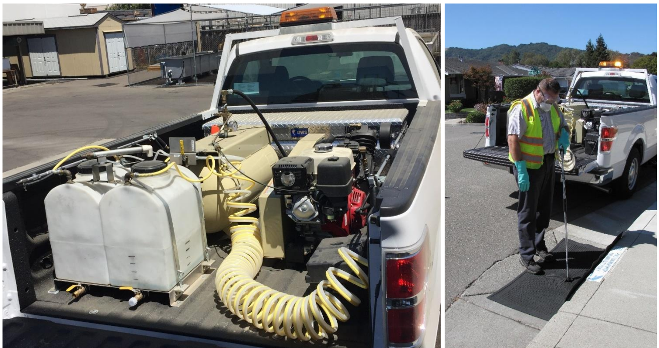
Figure 5. ULA mounted in the back of a District truck (left). District staff using the ULA to treat a catch basin for breeding mosquitoes.
